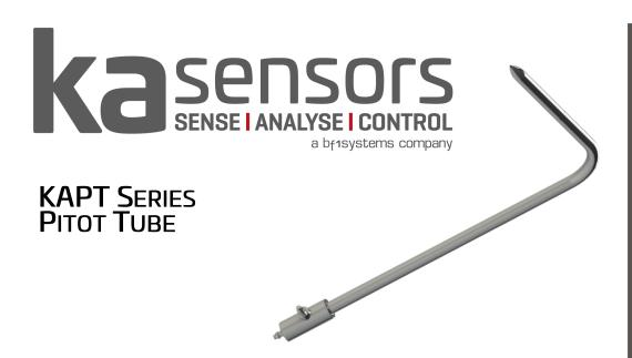
A Pitot Tube is used to measure Speed relative to the surrounding air. The assembly is made up of a pair of concentric tubes; the ellipsoidal nose cone at the tip has a small aperture in the end which is connected to the inner tube whilst an annular ring of holes on the outer tube senses the static/surrounding air pressure.
