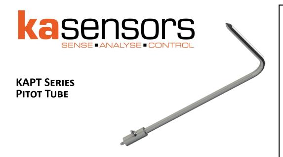
A Pitot Tube is used to measure Speed relative to the surrounding air. The assembly is made up of a pair of concentric tubes; the ellipsoidal nose cone at the tip has a small aperture in the end which is connected to the inner tube whilst an annular ring of holes on the outer tube senses the static/surrounding air pressure.
