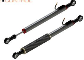
The KP Series of KP13S Standard Light Duty Linear Position Sensors are designed to withstand the harsh environments within motorsport and automotive testing applications. By using a proven conductive plastic, track technology and multi-fingered contacts, the KP13S offers high performance and reliability under extreme temperature and vibration.
