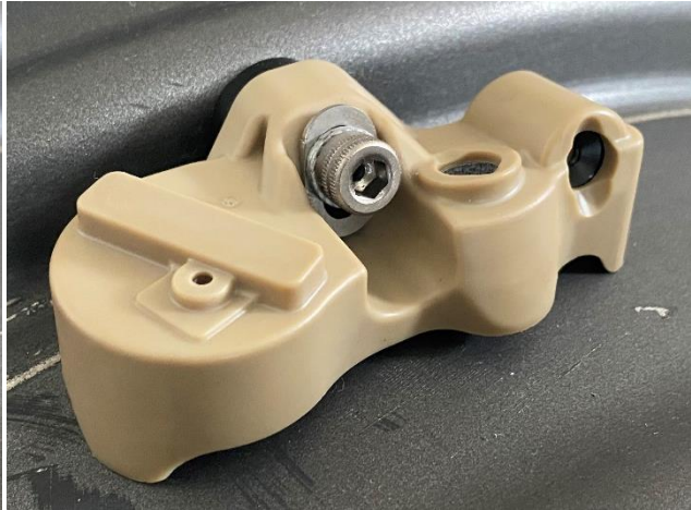
Figure 11 - 1SYSTEM® IRTPTMS Sensor
