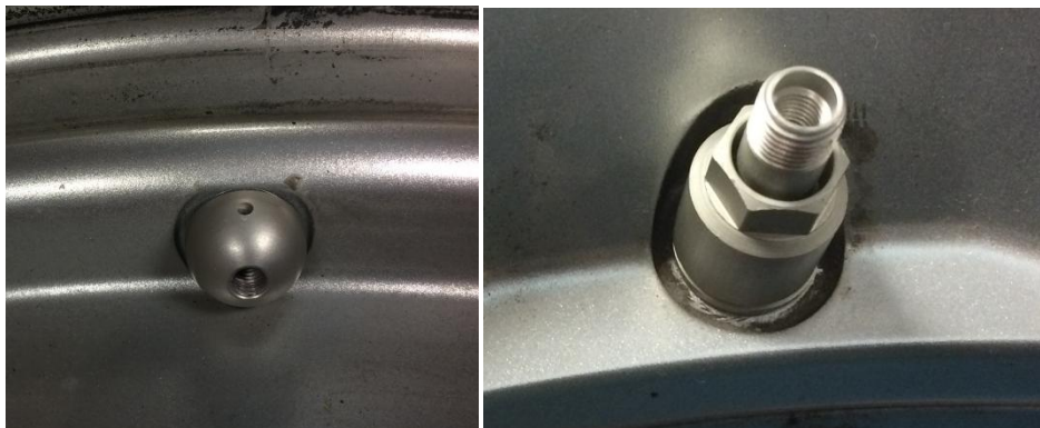
Figure 112 - Valve fitted to rim
