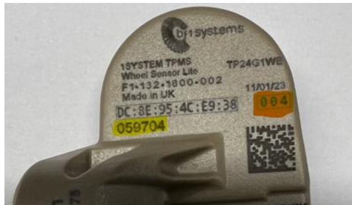
Figure 15 - Sensor Validation Code (highlighted in orange)
