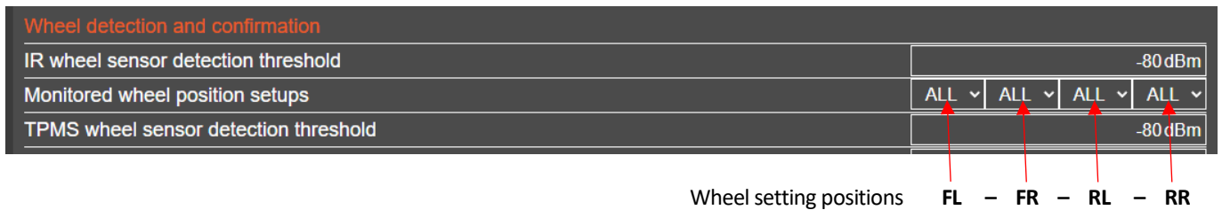
Figure 87 - Setting monitored wheel position
