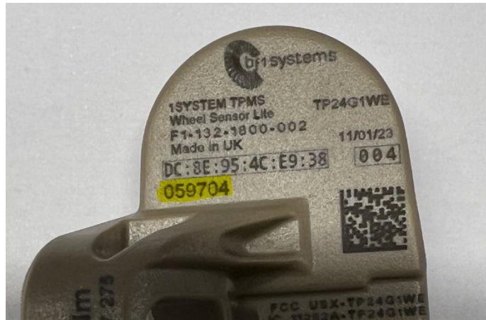
Figure 107 - 1SYSTEM® TPMS Wheel Sensor Serial Number
