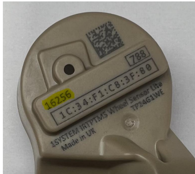
Figure 108 - 1SYSTEM® IRTPTMS Wheel Sensor Serial Number
