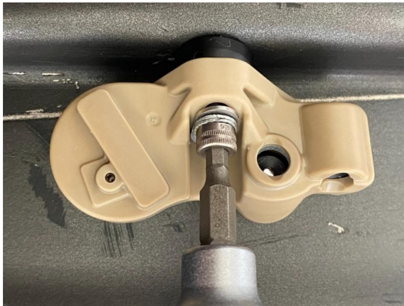
Figure 128 - Torque to 7Nm
