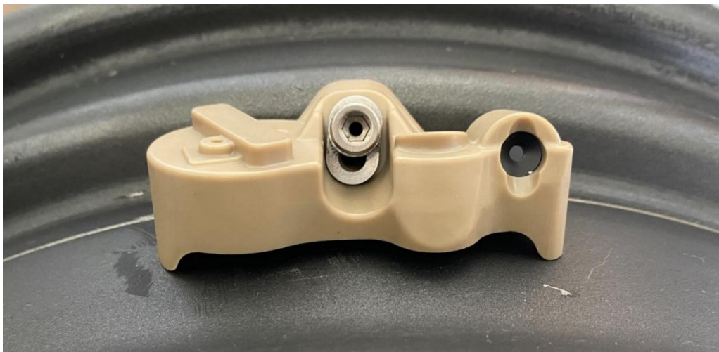
Figure 127 - IR sensor mounted on rim
