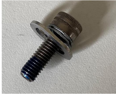
Figure 94 - Assembled screw with Loctite
