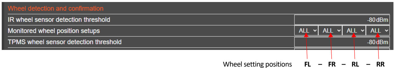
Figure 91 - Setting monitored wheel position
