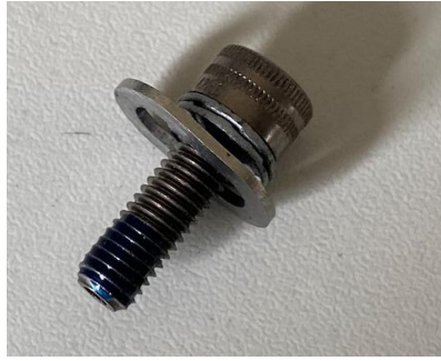
Figure 131 - Assembled screw with Loctite
